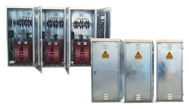
Cabinets with nominal voltage of 3.6 and 7.2 kV, intended for transformation centers with double (loop) supply, with cables up to 35 mm2 in section and a protected output.
